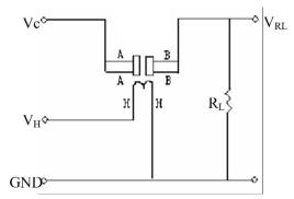
The above is basic test circuit of the sensor.
