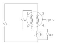
Calculation formula of sensor's consumption:  $Ps=Vc^2\times Rs/(Rs+R_1)^2$
