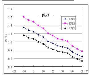
Pic2: Rs expresses the resistance under 1000ppmCH4 and various temperature and humidity conditions. Ro expressed the resistance under 1000ppmCH4 and 20°C/65%RH conditions.
