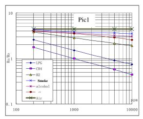
Pic1: Rs expresses the resistance of sensor in different concentration of gas. Ro expresses the resistance of sensor in 1000ppm CH4. All the tests in the picture are all finished under the standard testing condition.
